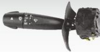
PROD. NO.: AI-456 A HEADLIGHT S/W UNIT ASSEMBLY
